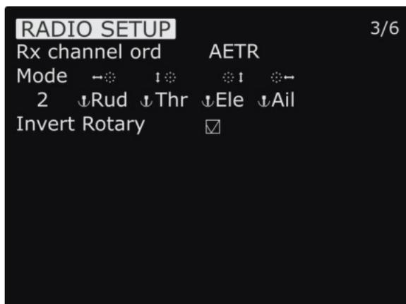
1. Long-press the Menu button to enter the Radio Setup
