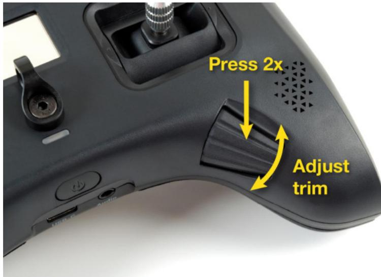
If you got a new airplane or wing, you can set up a special function to write the actual stick position to the trims by the push of a button. Details can be found [here](#).
