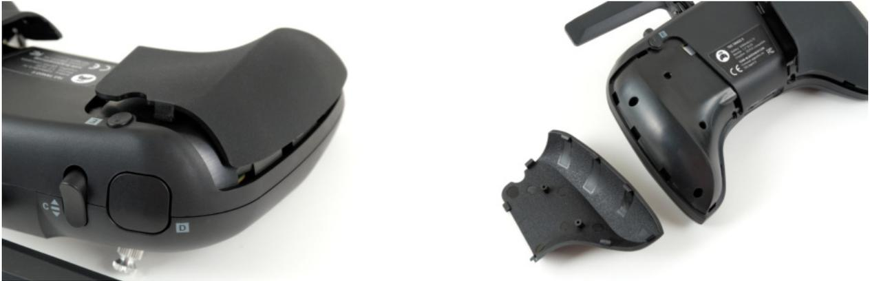
Then remove the six (6) screws, as indicated in the following photo with an M1.5 hex driver. Now, the back housing lifts off.
