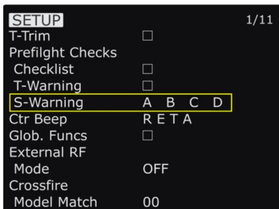
1. Press the Menu button and navigate with the PAGE button to the SETUP page
