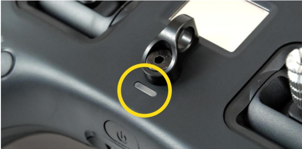
When the remote is powered on, the LED behind the button will show the actual status of the remote. The built-in LiPo battery is charged every time a 5V power source is connected to the USB-C connector.
