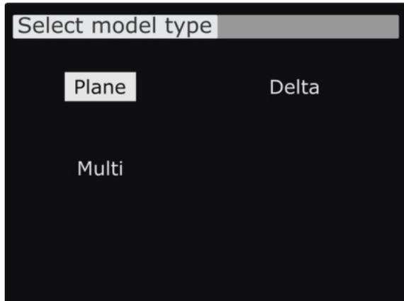
When creating a new model the wizard guides you through step-by-step. This can be aborted any time by pressing **EXIT**
