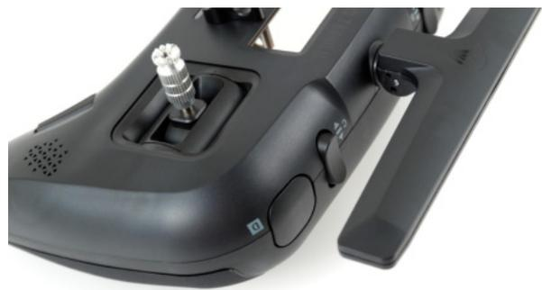
Right two-position (D/R1) switch and three-position (C/R2) switch
